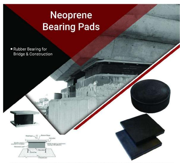
Black neoprene bearing pad is used as economical efficient bearing plates for pre-cast, pre-stressed concrete or steel beams in bridges and buildings. Neoprene Pads permit a smooth and uniform transfer of load from the beam to the substructure, allow beam rotation at the bearing due to deflection of the beam under load. They further allow lateral and longitudinal movement of the beam caused by thermal forces.
