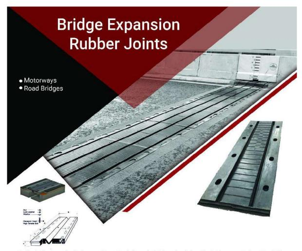
Rubber bridge expansion joints are mainly made of rubber, steel plate and angle iron. Steel plates are set in the rubber bridge expansion to strengthen the bearing capacity and they can slide freely along the angle iron to meet the expansion deformation of main grid.
